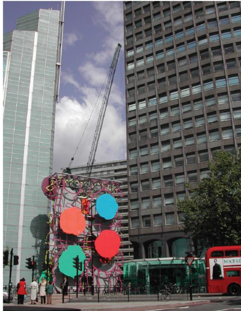
Figure 8: A wind sculpture used to provide wind shelter in a gap between two tall buildings
